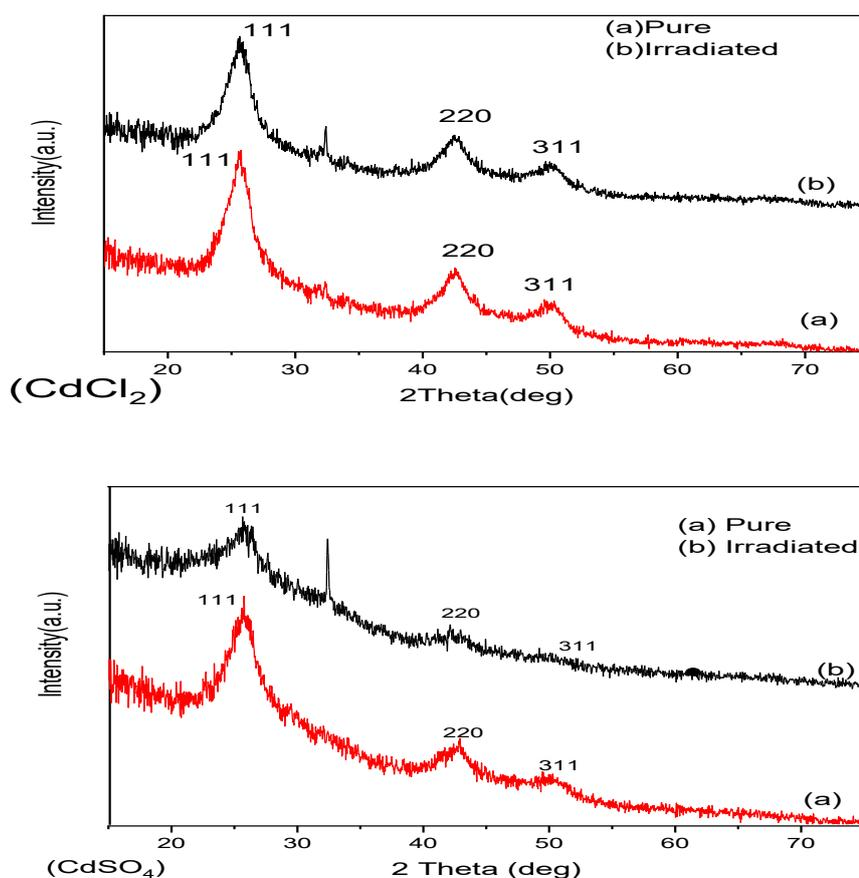
**Fig. 7:** X-ray spectrum of pure and irradiated CdSe films of two cadmium sources
