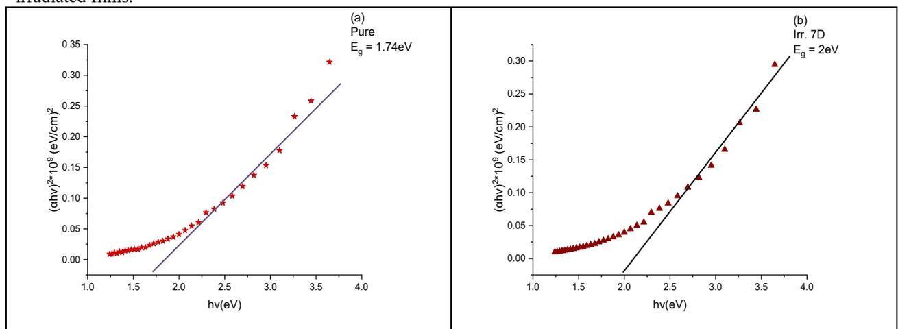
Fig. 3: energy gap of CdSe thin films :(a) pure (b) Irradiated
