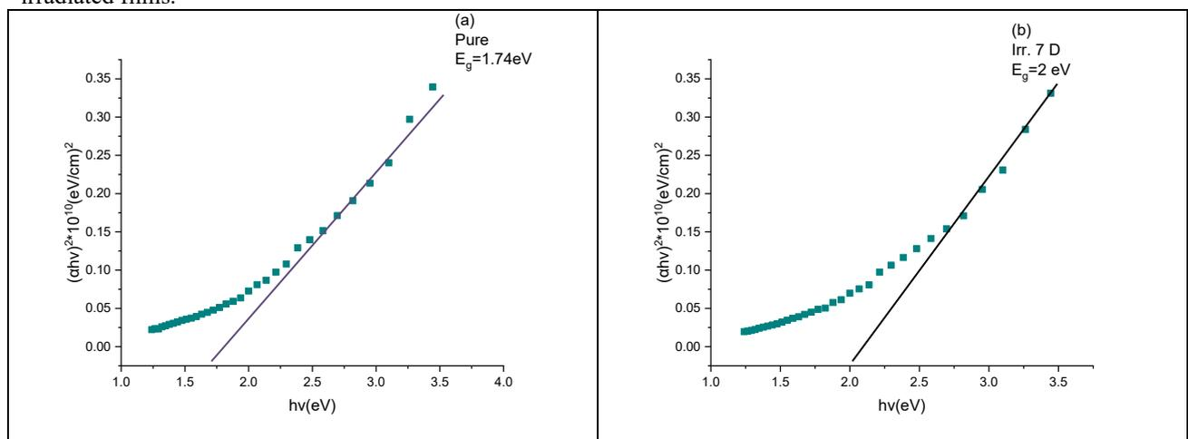
Fig. 2: energy gap of CdSe thin films :(a) pure (b) Irradiated
