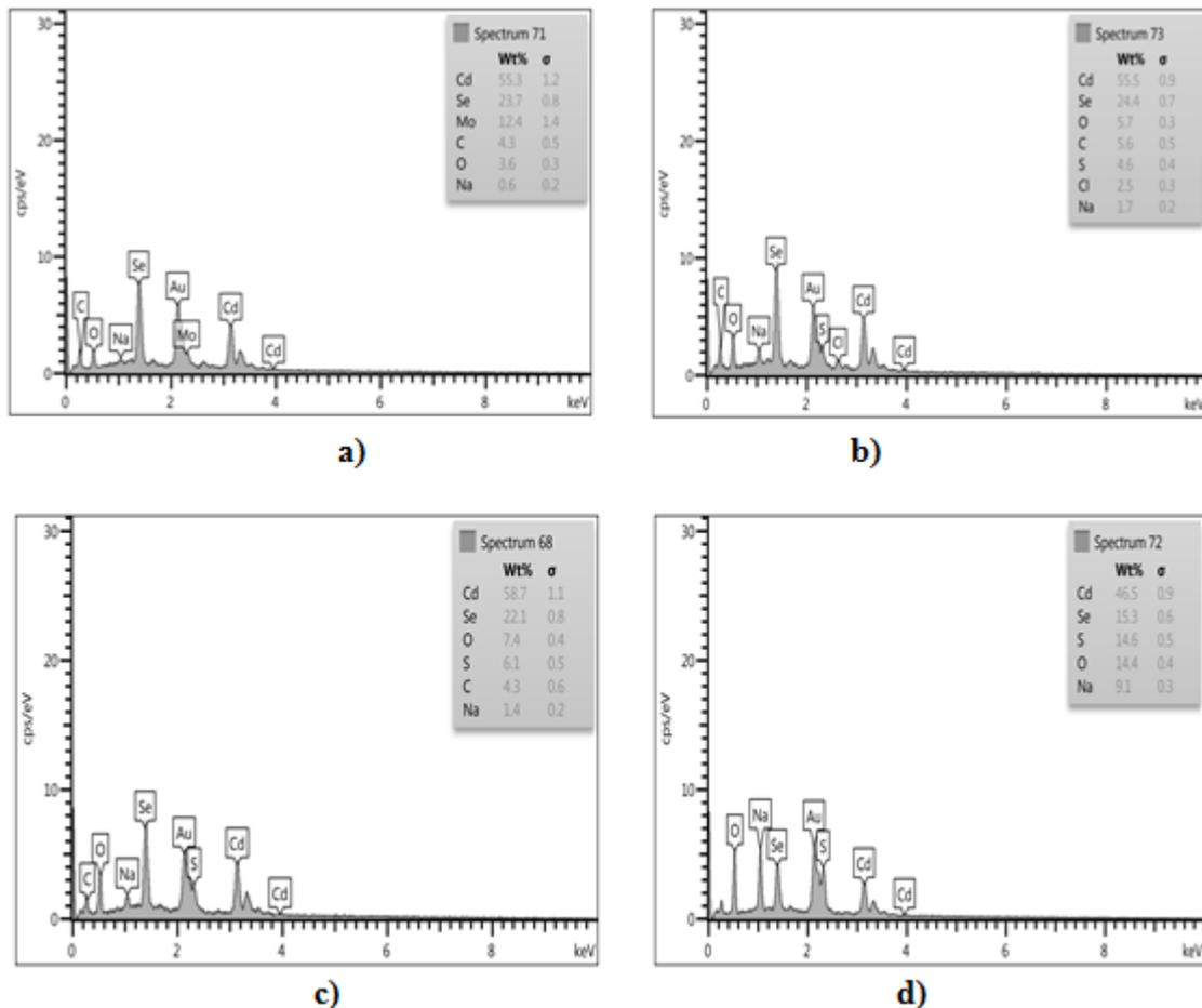
**Fig. 8:** The EDX pattern of CdSe films on the glass substrate for CdCl<sub>2</sub> material (a) pure (b) irradiated, for CdSO<sub>4</sub> material (c) pure (d) irradiated
