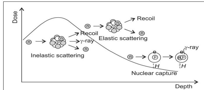
**Fig. 1:** Scheme of the interaction of neutrons with matter
