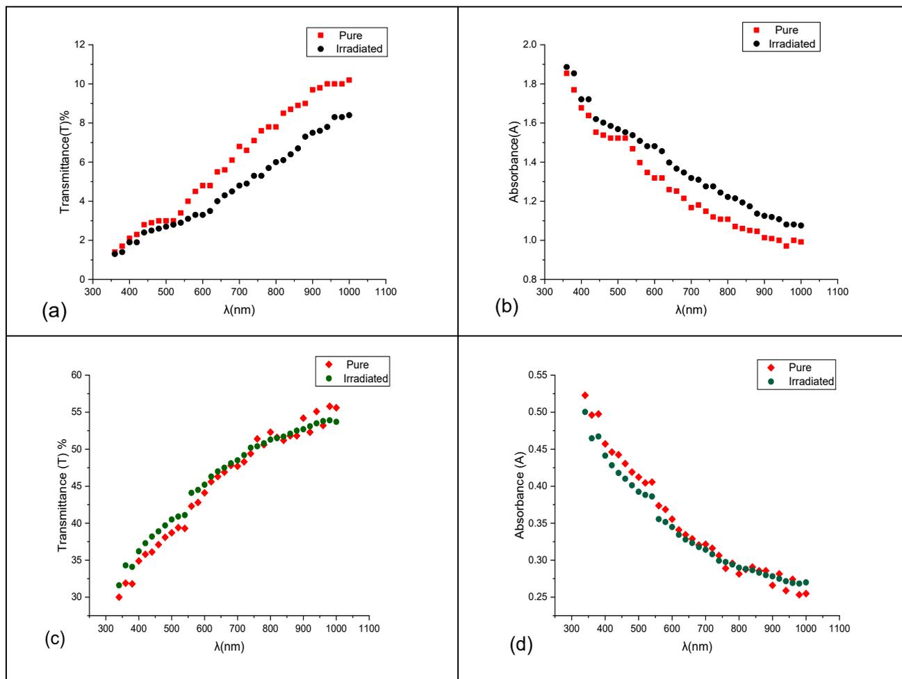
**Fig. 4:** Transmittance (T) and absorbance (A) as a function of wavelength ( $\lambda$ ) for pure and irradiated CdSe films:(a&b) for material CdCl<sub>2</sub> and (c&d) for material CdSO<sub>4</sub>
