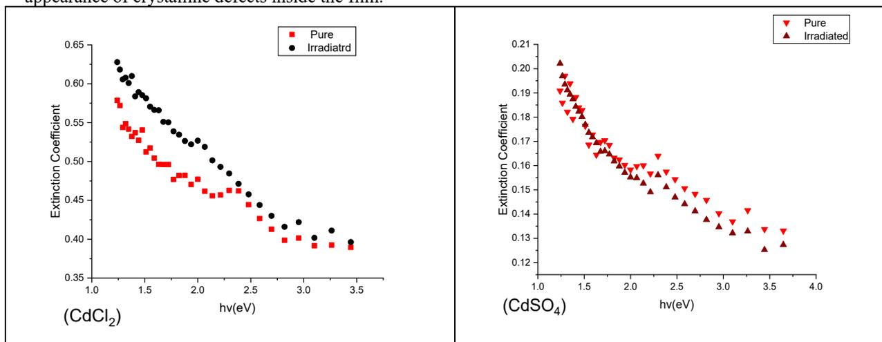
**Fig. 6:** The extinction coefficient (K) of CdSe films as a function of the photon energy before and after irradiation
